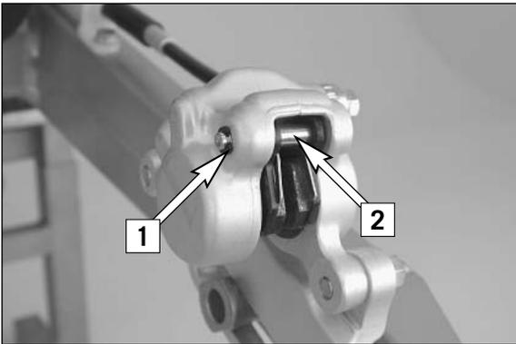
Remove the locking screw [1], unscrew the screw [2] and pull the brake shoes out of the brake caliper.
