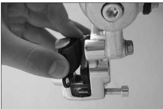
Mount the left brake shoe and fix with screw. Mount the right brake shoe and tighten the screw to 6 Nm. Mount the lock washer. Align brake shoes, mount front wheel (see chapter: Mounting the front wheel).
