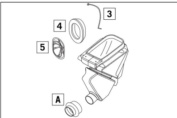
Thoroughly wash the foam filter in special cleaning fluid and allow to dry well. Only press out the filter, do not wring out under any circumstances. Oil the dry foam filter with a high grade filter oil. Also clean the air filter box. Check carburetor collar [A] for damage and that it is fitted correctly.
