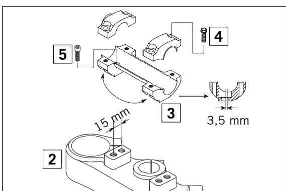
For this purpose, remove screws [4] of the handlebar clamps and screws [5] of the handlebar support. Position handlebar support, and tighten screws [5] to 40 Nm. Mount handlebar and handlebar clamps, and tighten screws [4] to 20 Nm. The gap between the handlebar support and handlebar clamps should be the same size in the front and in the rear.
