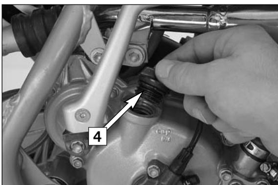
Remove the filler plug [4] and add 0.30 l gear oil 20W30 (e.g. Motorex Top Speed 4T 15W50). Mount the filler plug and check the engine for leaks.
