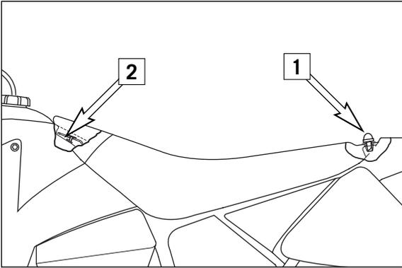
To mount the seat, position seat on the fixing screw [2] and tank, push forward and fix with the quick release.
