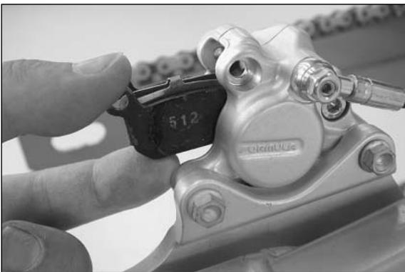
Slide new brake shoes into the brake caliper and fasten with the screw [2]. Tighten the screw to 4 Nm and mount the locking screw [1]. Mount the rear wheel and actuate the foot brake lever until you can feel the pressure point.
