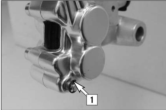
Remove the lock washer [1] from the screw as well as fixing screw [2] and take the brake shoes out of the brake caliper. Clean brake caliper thoroughly with compressed air.
