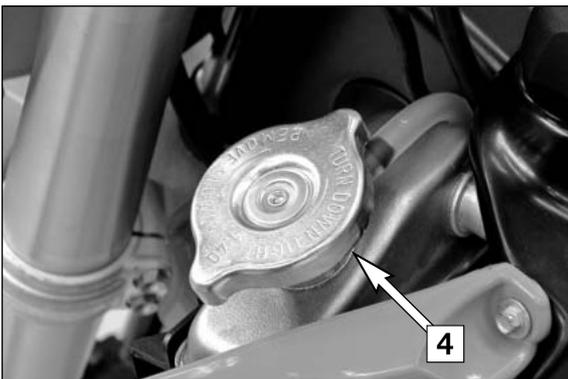
A mixture of 50% antifreeze liquid and 50% distilled water is used as coolant. However, the antifreeze protection must be at least  $-25^{\circ}\text{C}$  ( $-13^{\circ}\text{F}$ ). This mixture offers antifreeze protection but also good corrosion protection and should therefore not be replaced by pure water.
