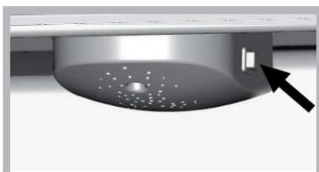
With the Active Oxygen switched on, the device will operate a repeated cycle until the key is pressed again. There will be an Ozone emission noticed by the switching on of the green led located on the Active Oxygen device located in the fridge compartment and a stand-by cycle (without ozone emission) noticed by blue light.
