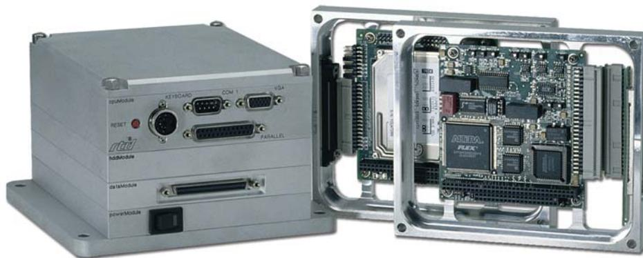
**IDAN**—Adhering to the PC/104 stacking concept, IDAN allows you to build a customized system with any combination of RTD modules.
