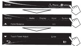
2 Touch the center of the marks at the lower left and at the upper right as instructed.
