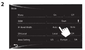
[Auto] Increases the tuner selectivity to reduce interference between adjacent stations. (Stereo effect may
