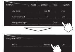
When < Input> is set to [iPhone], the [Apps] button is shown on the <HOME> screen, and the  $[\mathcal{A}]$  button is shown on the source control screen. You can display the App screen by pressing either button. (See the right column.)
