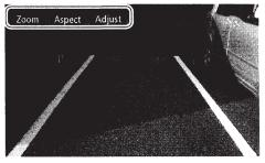
• When displaying the picture from the rear view camera manually, you can change the setting of the picture using [Zoom]/[Aspect]/[Adjust]. (Page 39)
