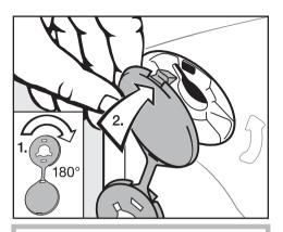
To avoid injury the holes for the shipping struts must be covered after the struts are removed.
