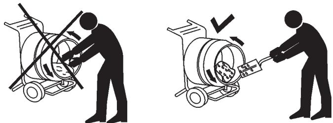
Figure 19. Mixing Drum (Placing Cement Mix)
