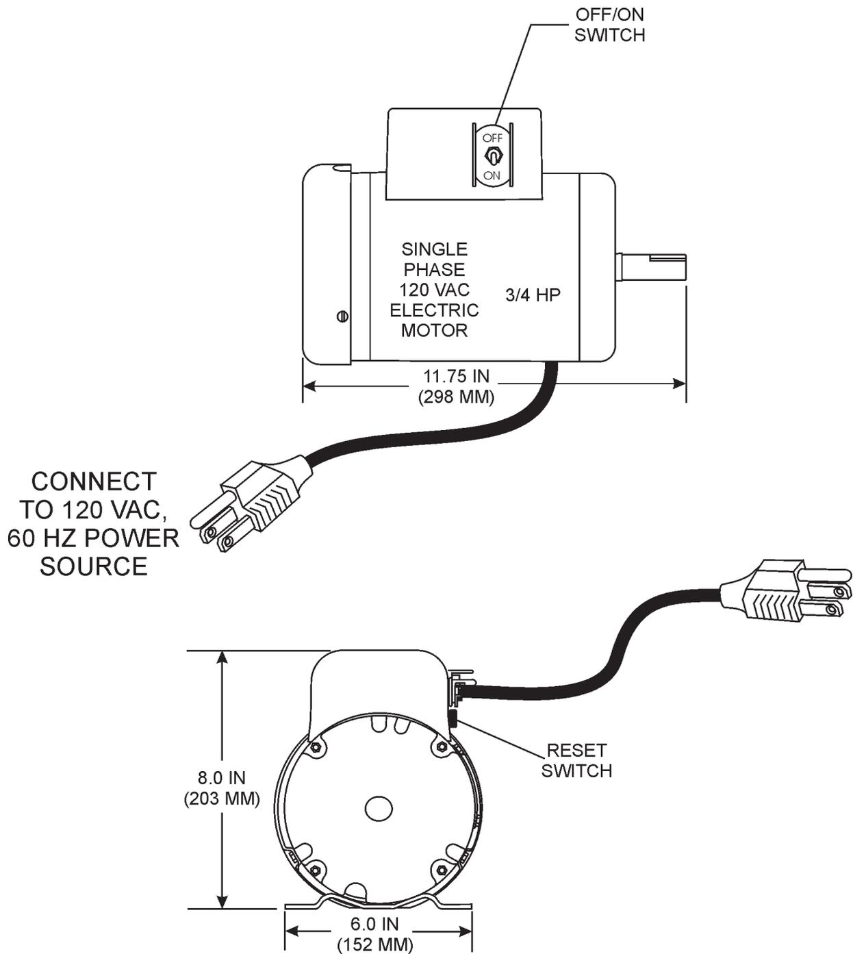
Figure 2. Electric Motor
