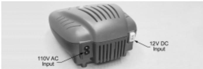
**WARNING** Never plug the charger into a 220V power source and never connect the charger to a 12V DC and a 110V AC power source at the same time. Use only one desired power source at a time. If connecting the charger to a 12V DC power source, make sure to attach the red alligator clip to the positive terminal and the black alligator clip to the negative terminal.
