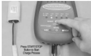
**IMPORTANT** If there is a battery error (i.e., reversed polarity or internal short), the charge rate LEDs will blink together shortly after you press the START/STOP button. If this occurs, remove the battery from the charger and check all connections and battery integrity before attempting to charge the battery again.
