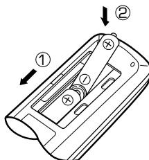
● Insert two AA-size (R6 / SUM-3) batteries as indicated by the polarity marking.
