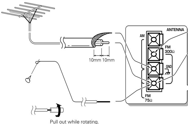
When using a commercially-available T-shaped indoor antenna (300 Ω), connect it to these terminals. (Remove the provided indoor antenna if you connect a T-shaped indoor antenna.)
