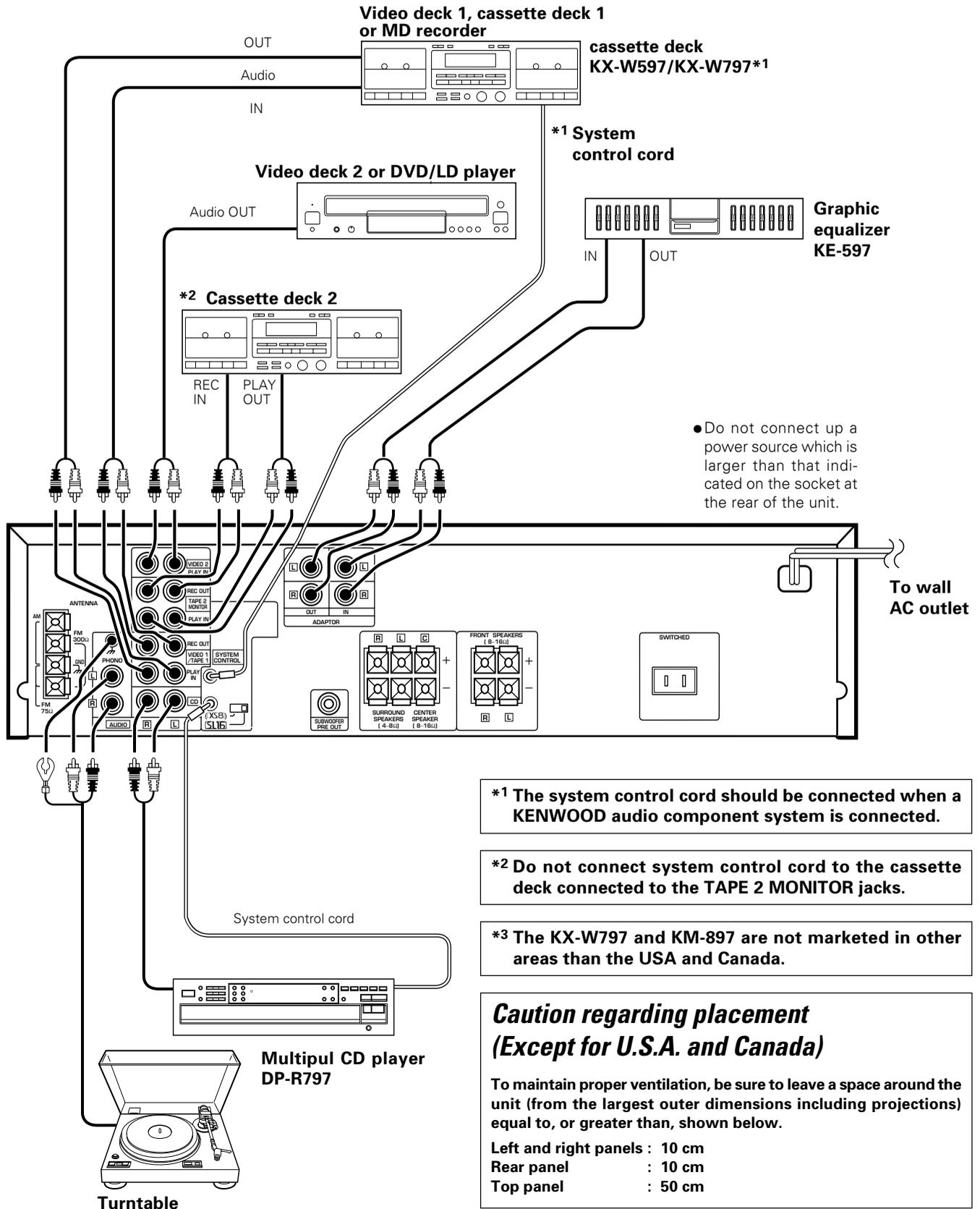
\*1 The system control cord should be connected when a KENWOOD audio component system is connected.
