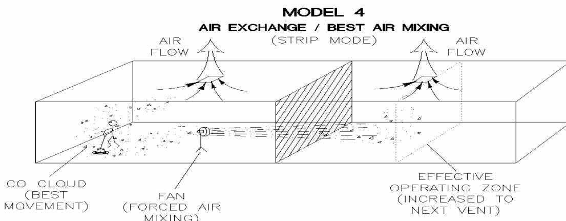
Notice the CO concentration and the Effective Operating Zone (Expanded through the Dividing zone to the second vent) with air exchange and forced air mixing through the dividing Zone. The CO cloud is diluted with the available air in the building. Note the "Dividing Zone" shown above, this is the line where airflow changes direction. In Model 4, air changes are full as forced air mixing has moved and mixed the CO between all air zones.
