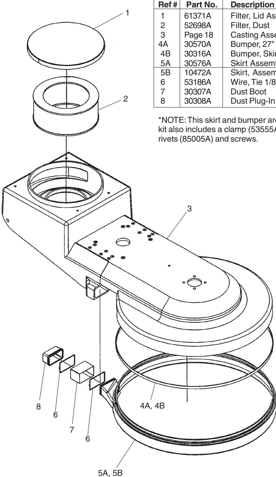
\*NOTE: This skirt and bumper are included in a kit (10861A). This kit also includes a clamp (53555A), two wire ties (53186A), and five rivets (85005A) and screws.
