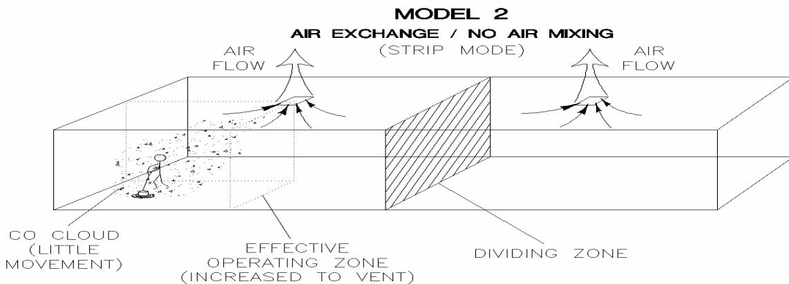
Notice the CO concentration and the Effective Operating Zone with air exchange. The CO cloud is still concentrated in a small area. Note the "Dividing Zone" shown above, this is the line where airflow changes direction. In Model 2, air changes are cut in  $\frac{1}{2}$  as little or no CO crosses the Dividing Zone to be exhausted.
