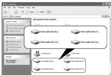
Drive letters for the removable disk icons are assigned in alphabetical order to the CompactFlash / Microdrive Slot, SmartMedia / xD-Picture Card Slot, MultiMediaCard / SD Memory Card Slot, and "Memory Stick" Slot.
