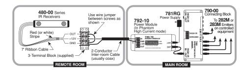
**CAUTION:** With any of these systems, be sure the 781 power supply is plugged into an un-switched AC outlet. This maintains the 480 system in "standby" operation so that power-on commands can be sent to the controlled equipment.
