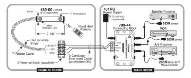
distant location, you may splice in 2-conductor wire, in the wire gauges mentioned before, as needed.
