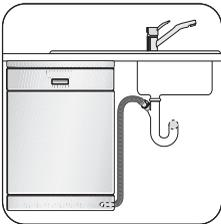
Connect drain hose to the sink. Secure it with the supplied hose clamp.
