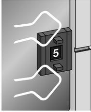
Note that in the case of a host computer which has a built-in SCSI hard disk or built-in CD-ROM, the ID numbers of the host CPU and each SCSI device have already been assigned.
