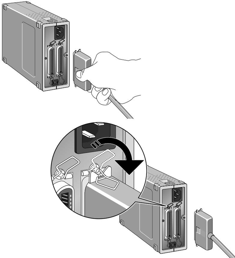
If the unit is the only connected SCSI device, or if the unit is connected at the end of the SCSI chain, attach a terminator (terminal resistance) to the other SCSI connector. At this point, remove the terminator of the other SCSI device that has been placed between them. The terminator is not needed when the unit is connected between other SCSI devices.
