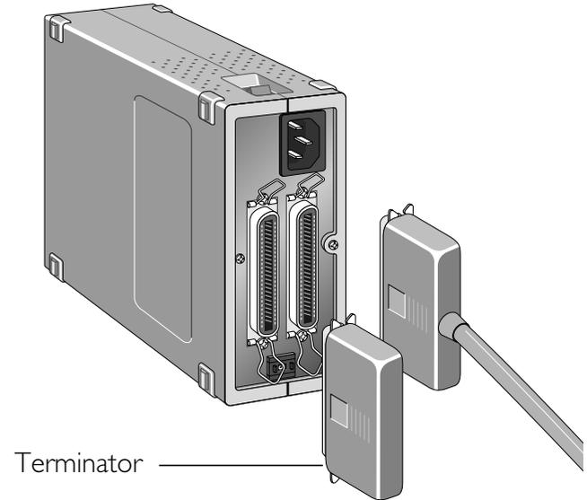
Connect SCSI devices in a chain, and attach terminators to both ends of the chain. Since the terminator is built into the host computer in most cases, the host computer should be at the end of the SCSI chain. The operation manuals of some notebook computers require a terminator to be attached outside the computer; please refer to the operation manual for the computer to which the unit is connected.
