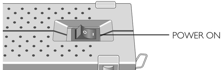
The scanner is self-calibrating. A calibration procedure occurs automatically during power-up. This procedure typically takes about twenty seconds.
