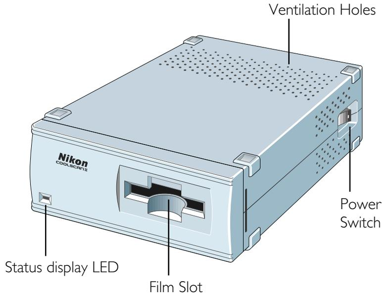
**Film Slot:** The film holder is inserted here.
