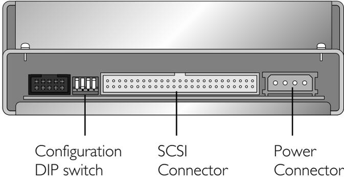
The default DIP switch configuration is shown in Table 5.1. The meaning of the SCSI ID DIP switch is explained later. The internal-mount scanner is set at the factory to SCSI ID #5.
