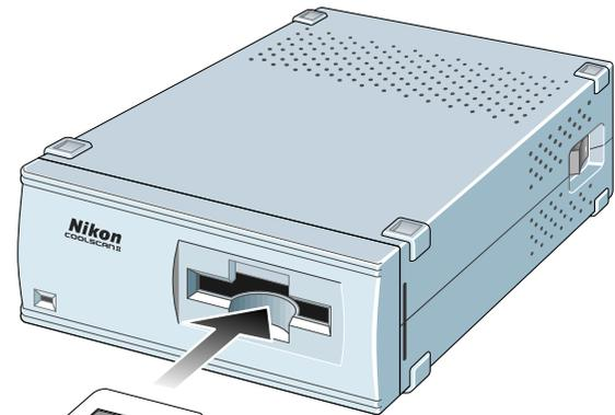
**Note:** Do not insert the mounted slide so that the width and length of the mount are reversed. If you do so, the COOLSCAN II will not be able to scan both sides of the mounted slide.
