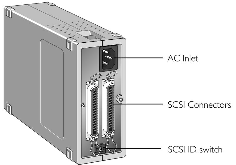
**SCSI Connectors:** For SCSI cable connection. No difference between IN and OUT.
