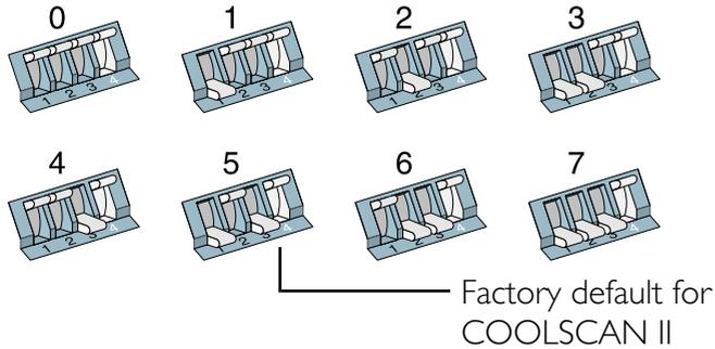
If it is necessary to change the default SCSI ID, change the position of the DIP switches to the proper SCSI ID. Refer to Table 5.2 for the proper DIP switch values. When changing the position of the switches, use a pointed instrument to toggle the switch. Use of a pen or pencil is not recommended, since these will leave a mark on the switch and make it difficult to differentiate between the “on” and “off” positions.
