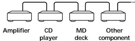
In the CONTROL A1II control system, the control signals flow both ways, so there is no distinction of IN and OUT jacks. If a component has more than one CONTROL A1II jack, you can use either one, or connect different components to each jack.
