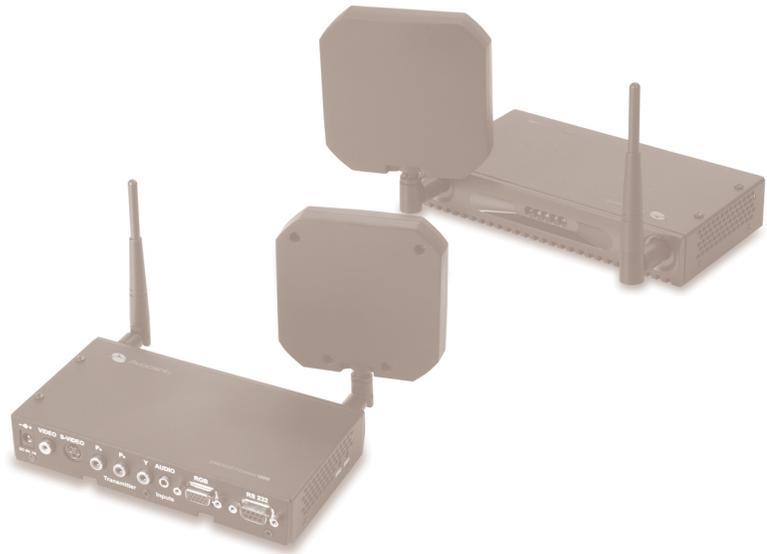
Transmitter and receiver pair with properly aligned antennas
