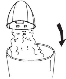
The dust bag/filter must be cleaned from time to time to remove the fine dust particles that have been collected. This can be done by either shaking it or for a more thorough clean, rinsing in cold water.
