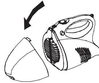
Pull out the dust bag/filter, by grasping the side of the filter and pulling out.
