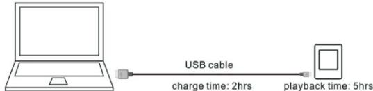
The Digital Photo Keychain battery is charged using the USB cable. Simply plug the USB cable from an available USB port on your computer or USB hub into the USB jack on the Digital Photo Keychain. Charge the Digital Photo Keychain for approximately 2 hours for full charge. At full charge, the Digital Photo Keychain provides up to 5 hours of photo playback enjoyment.
