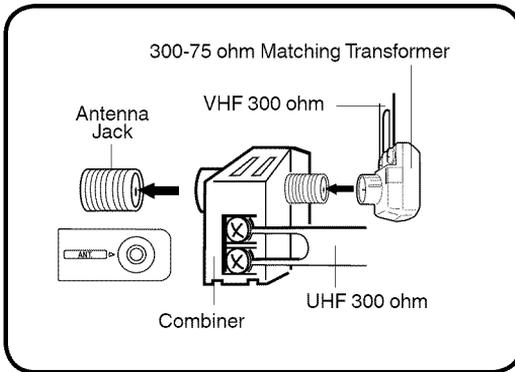
Connect the UHF 300 ohm twin-lead wire to the Combiner (not supplied). Connect the VHF 300 ohm twin-lead wire to the 300-75 ohm Matching Transformer. Attach the Transformer to the Combiner, then attach the Combiner to the Antenna Jack.
