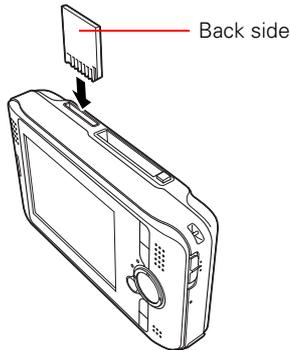
To remove a card from the SD Card slot, first make sure the Access light is off. Then press in on the top of the card.
