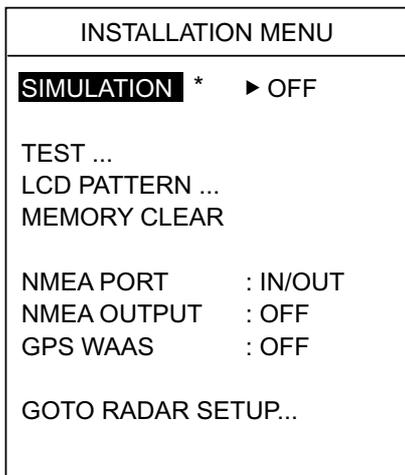
\* The simulation provides internally generated echoes, for use in exhibitions, etc. "SIM" appears at the top left corner when the simulation mode is active.
