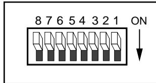
Figure 2-1. Default Mode Switch Settings (All Switches OFF)
