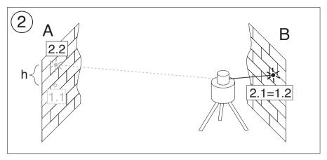
If the unit is within its working accuracy limits (± 20") the maximum difference from true level at 20 m (65 ft.) + 20 m (65 ft.) = 40 m (130 ft.) is 4 mm (3/16 inch).
