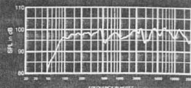
FIGURE 1 Axial Frequency Response, 4-Volts/10 Feet
