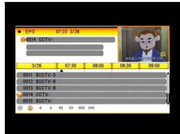
**3. Detail Information:** In the **EPG** window, press **PR+**, **PR-**,  $\leftarrow$   $\rightarrow$  keys to select the channel and program, and press **OK** key to know the detail information of the current program.
