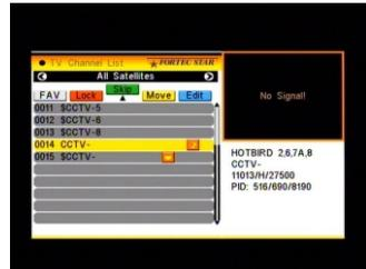
6. Press **yellow** colour key to move the Move button upward. Select the program and press **OK** key to mark this program with the move mark. Press **PR+**, **PR-** keys to move the cursor to the position where you want to locate and press **OK** key to confirm.
