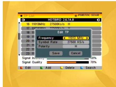
**Polarity:** Press  $\leftarrow$   $\rightarrow$  keys to switch between Vertical and Horizontal.
