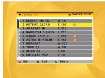
3. Press **red** colour key to pop up the **Edit Satellite** window. Press **PR+**, **PR-** keys to move cursor up or down.
