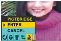
4. Connect your camera to a PictBridge compatible printer until you see a message "Pictbridge PRINTING", and do not unplug the USB cable until the message disappear on the screen.
