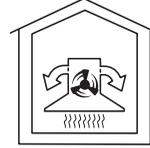
Air is drawn through the grease filters and an **active charcoal filter**. The filtered air is then recirculated back into the kitchen through a vent at the top of the hood's chimney.
