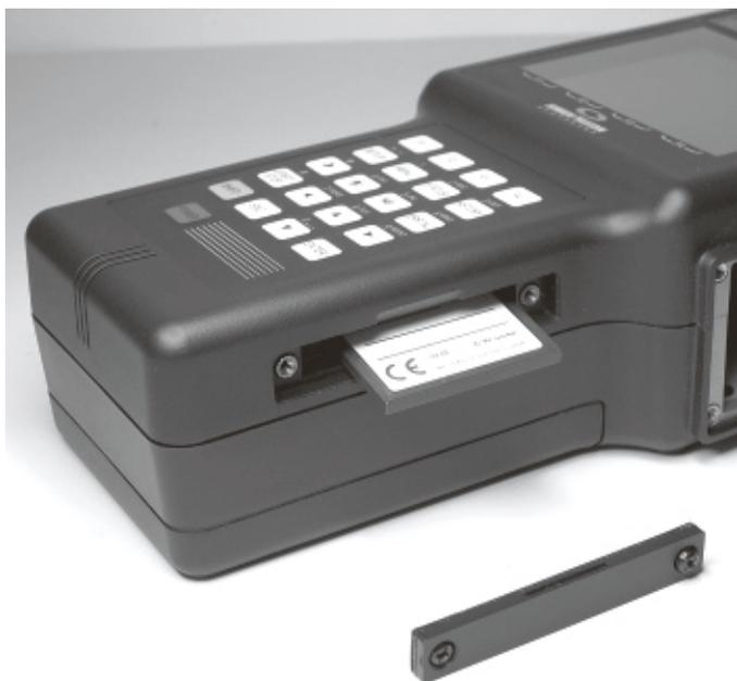
Insert the new memory card and press it firmly but gently into the slot. Replace the protective cover. Powering the unit on will automatically load the new software into the CM1000. This process may take several minutes depending on the software being loaded. The Link LED will flash green during the software update process.
