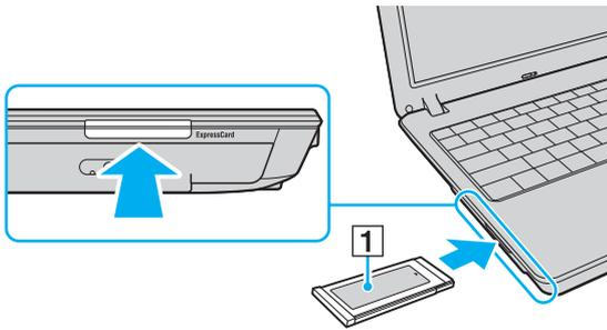
! Insert the ExpressCard slot protector to protect against debris entering the slot when not using an ExpressCard module. Before moving your computer, make sure to insert the ExpressCard slot protector into the slot.
