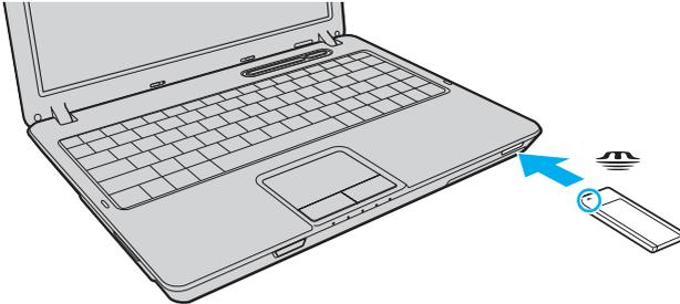
! Be sure to hold the Memory Stick media with the arrow pointing in the correct direction as you insert it into the slot. To avoid damaging your computer or the Memory Stick media, do not force the Memory Stick media into the slot if you cannot insert it smoothly.
