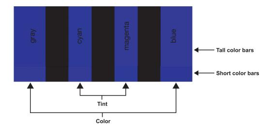
**Tint:** Tint or "hue" is essentially the ratio of red to green in the color portion of the image. When tint is decreased, the image appears redder; when it is increased the image appears greener. To set the tint, select Tint from the Picture Adjust menu. While looking at the color bar pattern through a blue filter, adjust the tint level until the cyan and magenta color bars (on either side of the green bar) appear to be a single shade of blue.
