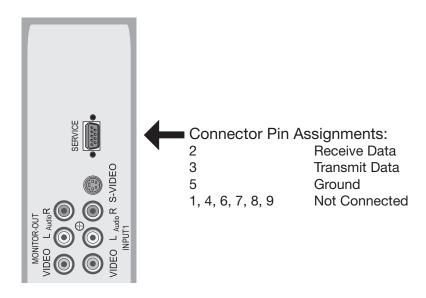
Figure 3-8. RS-232 Control System Connection
