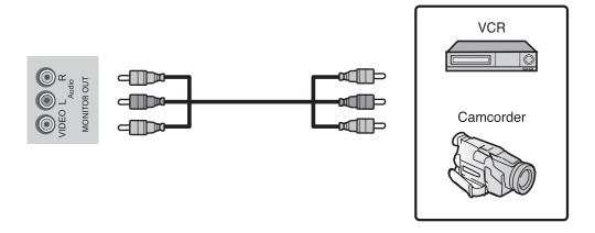
Figure 3-6. Monitor Output Connections
