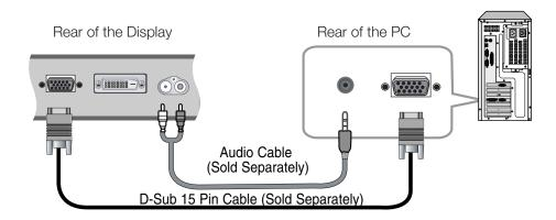
Figure 3-3. Analog RGB Connections
