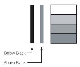
Figure 4-2. Typical PLUGE Pattern for Adjusting Brightness
