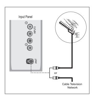
Figure 3-1. Antenna/Cable TV Connection
