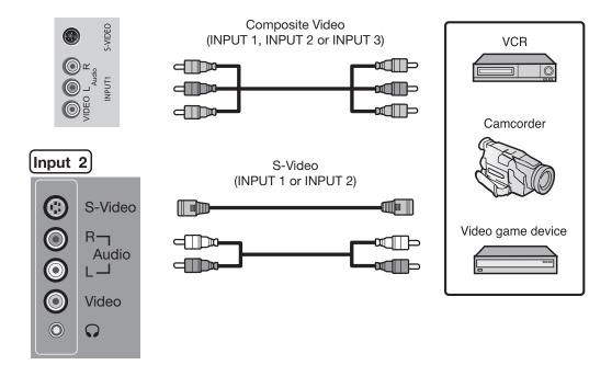
Figure 3-5. Composite and S-Video Connections
