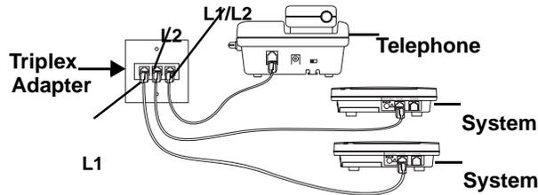
1. Disconnect the telephone line cord from the modular phone jack (on the wall) and plug it into **L1 + L2** on the triplex adapter.
