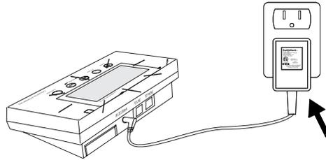
To power the system, plug the adapter's barrel plug into the **9V DC 200mA** jack on the back of the system. Then connect the other end of the adapter to a standard AC outlet.
