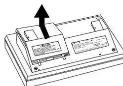
**Caution:** The battery compartment cover is attached to the system. Do not try to remove it completely.
