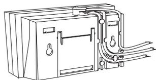
6. Line up the keyhole slots on the bracket with the screws in the wall, then slide the system down onto the screws until it is secure.
