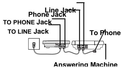
1. Disconnect the phone line cord that connects your answering machine to the phone line from the answering machine's jack. Then plug it into the system's **TO LINE** jack.
