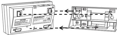
1. Align the keyhole slots on the bottom of the system with the hooks on the mounting bracket.
