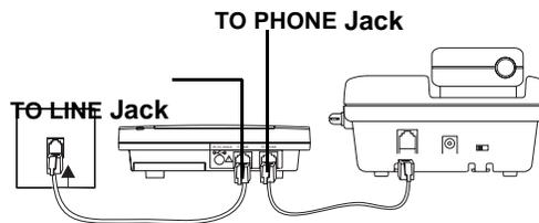
1. Disconnect the telephone line cord from the phone and plug it into the system's **TO LINE** jack.
