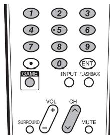
When you press **GAME** on the remote control unit, the input from INPUT 1 or INPUT 4 terminal is automatically selected and displayed on the TV screen at the optimum speed. You can toggle INPUT 1 and INPUT 4 by pressing **GAME** on the remote control unit. Press **CH**  $\wedge/\vee$  or **0-9** when you want to switch back to the TV.
