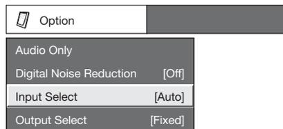
**4** Press **▲/▼** to select the equipment connected to INPUT 7 terminal, and then press **ENTER**.
