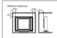
If the television is to be built into a compartment or similar enclosure, the minimum distances must be maintained. Heat build-up can reduce the service life of your television, and can also be dangerous.
