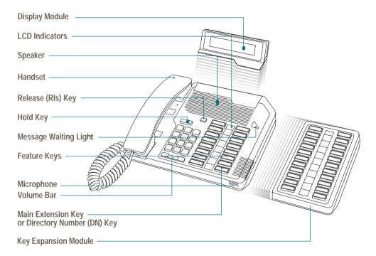
The M2006 has six feature keys; the M2008/M2008HF has eight feature keys; the M2616, shown above, has 16 feature keys and a built-in microphone.
