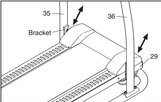
**CAUTION:** Make sure that the incline knobs are fully inserted at the same height.
