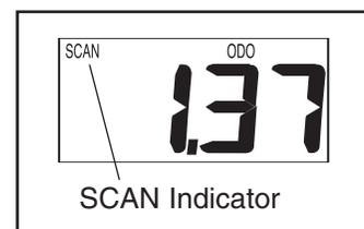
To select only the Speed, Distance, Time, Odometer, or Calorie mode, press the console button until only the SPEED, DIST, TIME, ODO, or CAL indicator appears in the display. Make sure that the SCAN indicator does not appear.
