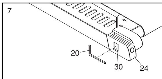
8. **Make sure that all parts are properly tightened before you use the treadmill.** To protect the floor or carpet, place a mat under the treadmill.
