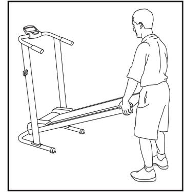
2. Hold the treadmill securely with your right hand as shown. Insert the Storage Pin (4) into the hole in the left side of the Left Upright (35) and into the Frame (29) as far as it will go.
