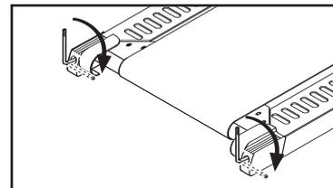
of a turn. When the walking belt is correctly tightened, you should be able to lift each side of the walking belt 5 to 7 cm (2 to 3 in.). Walk on the treadmill for a few minutes. Repeat until the walking belt is properly tightened. Be careful to keep the walking belt centred.
