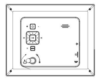
**Attaching the stand:** screw in the stand clockwise until it is secure. **Removing the stand:** unscrew the stand counter-clockwise until it is detached.
