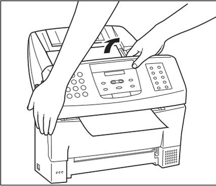
**2** While holding the operation panel open, pull the sheet out from the top or bottom.
