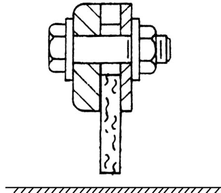
The poly blade should come as close as possible to the surface without touching. If material builds up on the drum, you may use a rubber mallet to dislodge the material without adverse effect to the drum.
