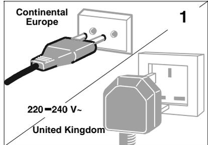
The plug is fitted with a fuse which protects your television. If your television does not work, the fuse may be blown. In this case, replace it with an identical 5 Amp ASTA or Ir BSI (BS 1362) certified fuse.
