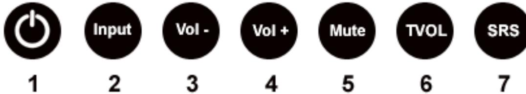
1. **Power** – Use this button to turn HD Sound Bar System ON or OFF.
