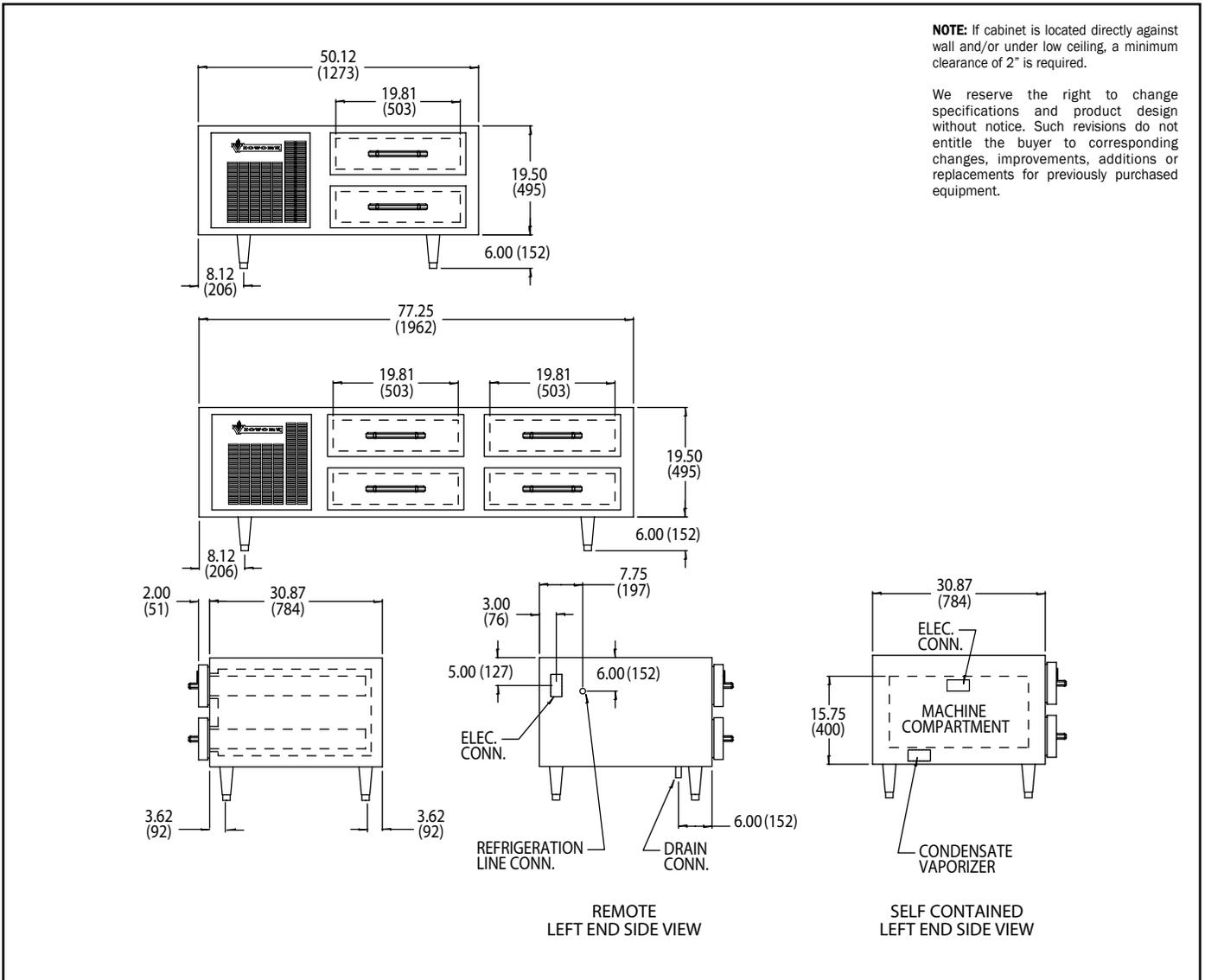
**NOTE:** If cabinet is located directly against wall and/or under low ceiling, a minimum clearance of 2" is required.
