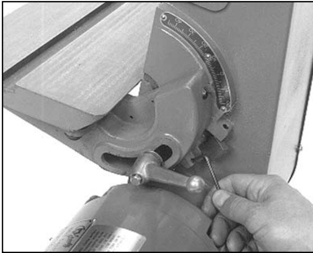
Figure 10. Adjusting belt table stops.
