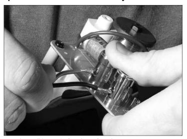
Strip about ½" (13 mm) of insulation from the connecting wires. Connect them to the appropriate push terminal, being careful to observe polarity (positive to the red terminal, negative to the black terminal).
