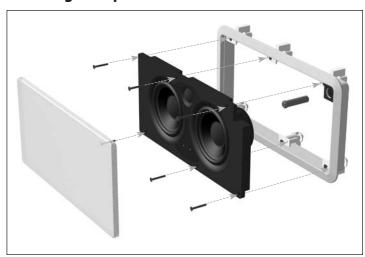
Once the frame is mounted in the wall, the speaker simply fits into the frame. Note that there is a gasket around the edge of the MDF baffle. This gasket ensures an airtight fit between the baffle and the frame. Therefore, the baffle may fit tightly in the frame. This is normal.
