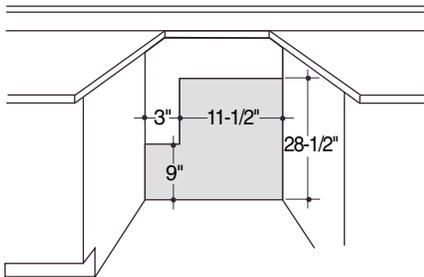
Electrical Supply Should Enter From Back Wall In Shaded Area.
