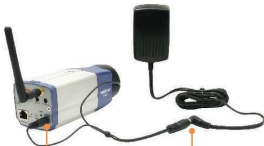
4. Connect the AC Power Adapter to the Internet Camera and then to a power outlet.
