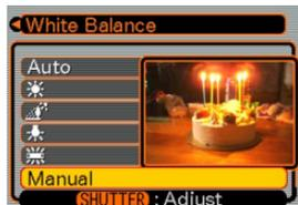
4. Point the camera at a white piece of paper or similar object under the lighting conditions for which you want to set the white balance, and then press the shutter release button.
