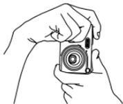
When holding the camera vertically, make sure that the flash is above the lens. Hold the camera still with both hands.
