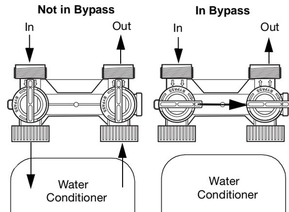
Figure 1 - Autotrol Series 1265 Bypass Valve
