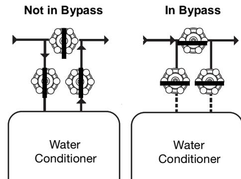
Figure 2 - Typical Globe Valve Bypass System
