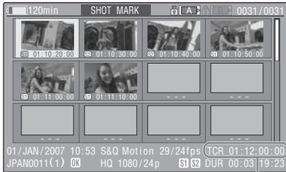
The detailed information of the clip is displayed at the bottom of the screen.
