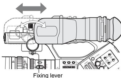
Tighten the fixing lever after the adjustments.
