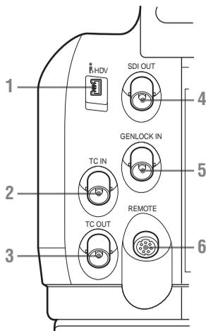
1. **i.LINK (HDV) connector (4-pin, S400 conforming to IEEE1394)** (page 135)
