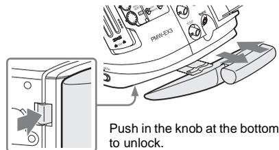
Push in the knob at the bottom to unlock. Hold the knob depressed when pulling out or pushing in the pad.
