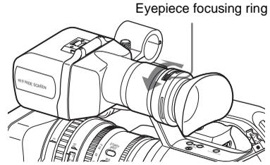
You can also attach a commercially available 52-mm aperture diopter compensation lens.
