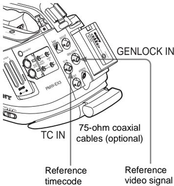
Thus the built-in timecode generator of your camcorder locks to the reference timecode. The message “EXT-LK” is displayed on the screen.
