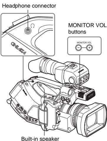
With the headphones connected to the headphone jack, the built-in speaker is turned off.
