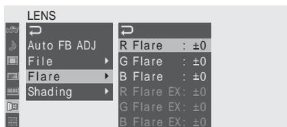
(Set the items with “EX” when a lens extender is in use.)
