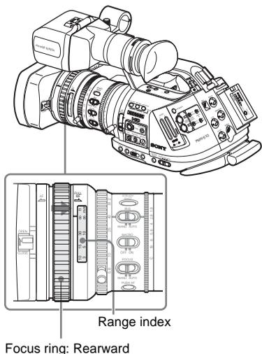
Rotate the focus ring for the best focus while observing the picture in the viewfinder. The range index of the focus ring is effective in Full MF mode. The distances correspond to the focus ring positions.
