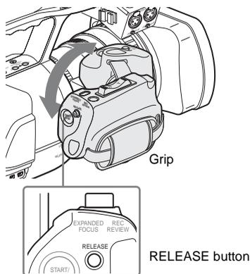
Click positions are provided at each 15 degrees. Release the **RELEASE** button at the desired click position to lock the grip.
