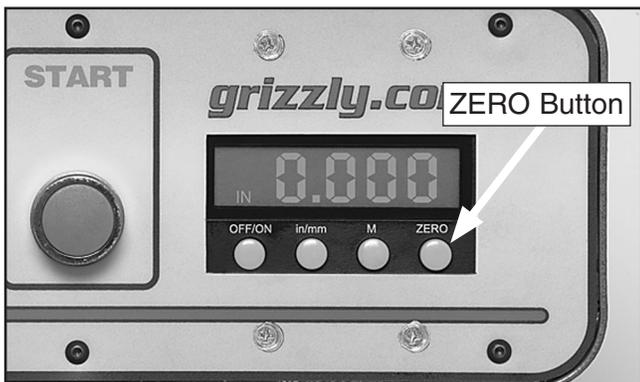
**Figure 59.** Digital readout zero button.
