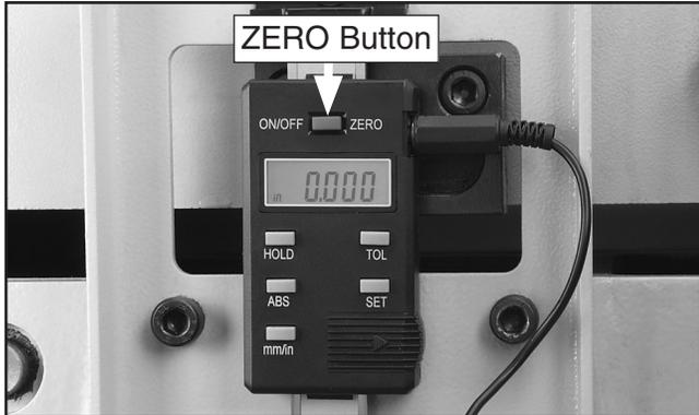
**Figure 58.** Sensor zero button.
