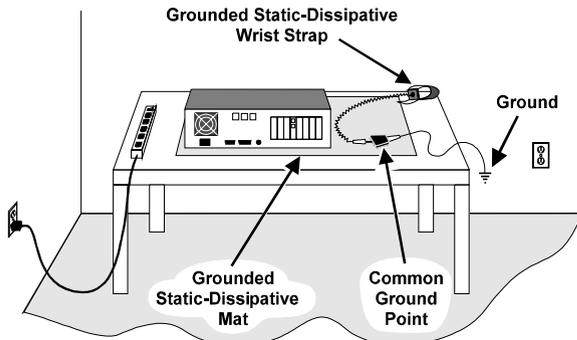
The work surface drains electrical charges from conductive materials when the materials are placed on the surface. The grounded, static-dissipating wrist strap drains static charge from the person wearing the strap. Both components ensure that static charges are drained at a rate and current level that are safe. Both must be used any time a person is handling a board or component.
