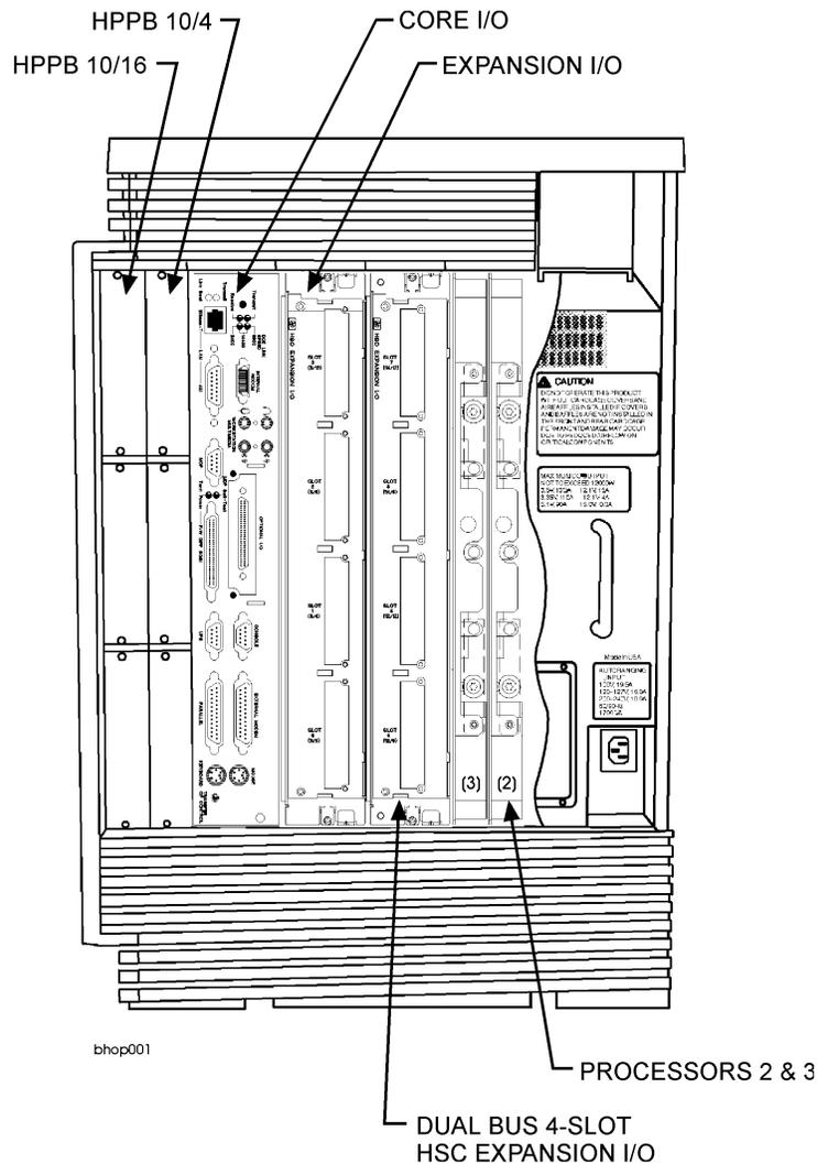
7. Remove the adjoining processor slot's cover plate by loosening the two (one top and one bottom) captive mounting screws and pulling the cover plate away. (This is necessary to gain access to the system board.)
